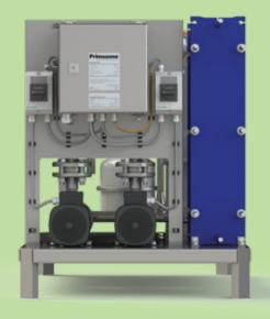
The ozone generators need cooling. If cooling water is available on site, Primozone CSM, cooling skids module, with heat exchanger and circulation pumps, are normally the preferred solution. The cooling skid makes a closed loop, with the ozone generator(s) on one side and the cooling water on the other, and there for preventing water, not clean enough, reaching the ozone generator(s). With a closed loop and a cooling skid the risk of damaging the ozone generator(s) is more or less eliminated.
